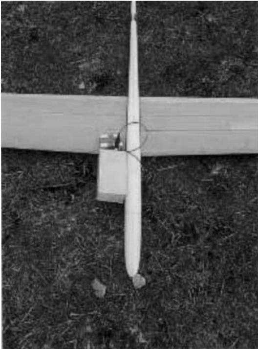
**Figure 18-4** Glider with camera pointing downward.
