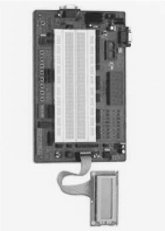
**Figure 1-7** Parallax NX1000 protoboard.
