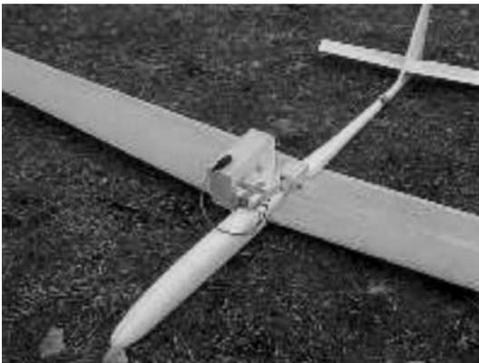
**Figure 18-5** Glider with camera pointing sideways.
