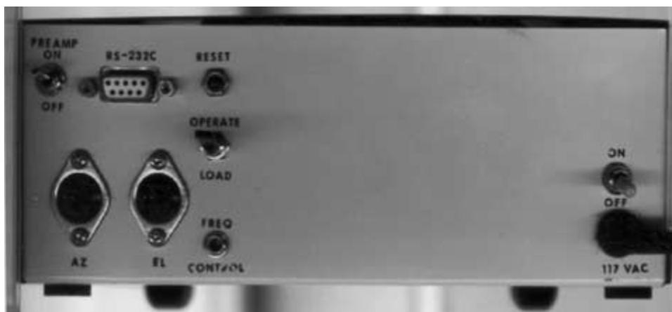
**Figure 15-3** Orb-Tracker chassis panel.
